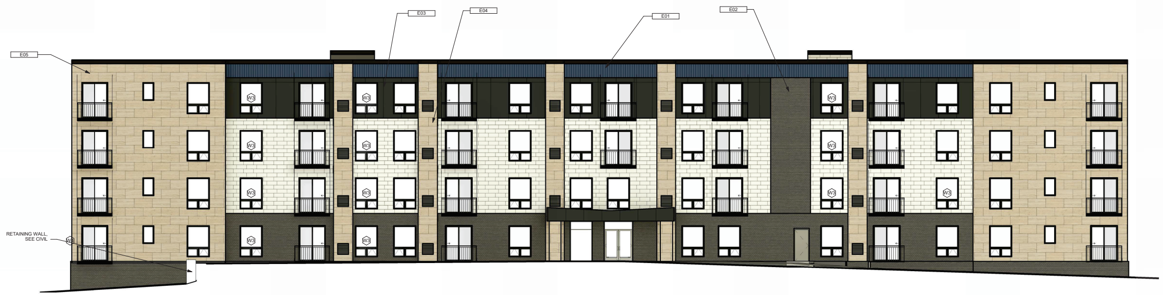
1 EXTERIOR COLOR ELEVATION NORTH A411 1/8" = 1'-0"
